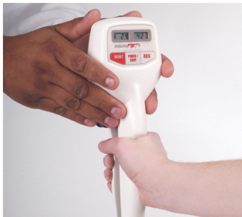
Figure 6.1 The microFET4 dynamometer is used for quantifying grip strength.
